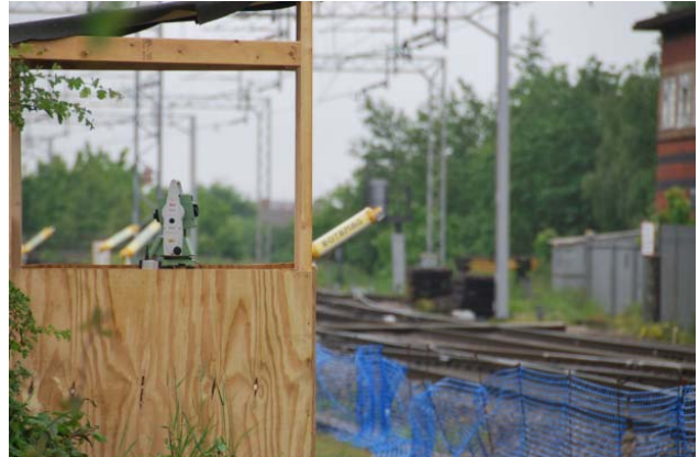
Pictured below: One of the two Leica TPS1200+ Total Stations measuring automatically to the mini prism at predetermined intervals, 24 hours a day.
